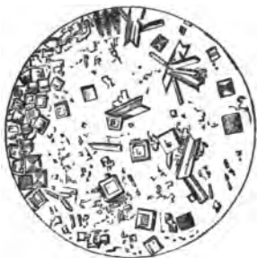
FIG. 13.—What is seen when a drop of concentrated sea-water is evaporated under a microscope.
